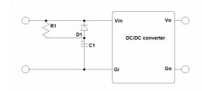
R1 = Power resistor to limit inrush current
